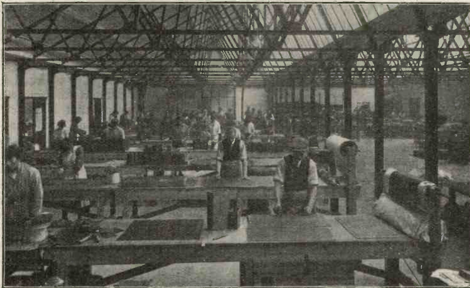
By courtesy of Messrs. Fullers United Electric Works, Ltd. Ebonite making-up shop. Note the raw dough in sheets and in rolls with linen to prevent the surfaces from sticking.
