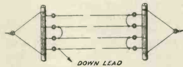
Fig. 3.—The wrong way to arrange the wire in an indoor aerial of small size.
